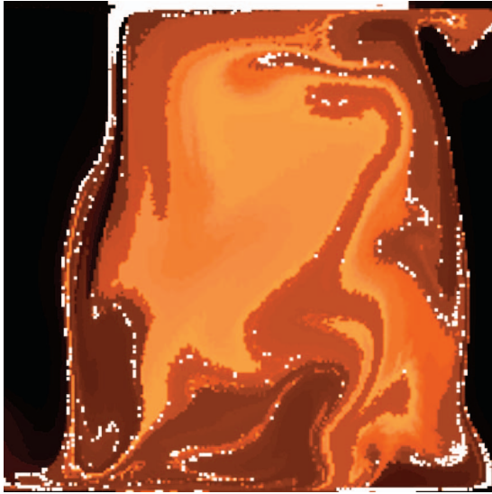
FIG. 6. (Color) Color-coding of the residence time of particles of the box shown in Fig. 4. Depending on how long it takes for the particles to leave the box (how long it takes to mix with the surroundings), the initial positions are colored differently: black colors toward dark red denote initial positions wherefrom particles escape very rapidly; light red toward white mark initial positions where particles tend to stay a long time within the box. White colors denote places wherefrom particles do not leave the box during the simulation time (ten overturns).
