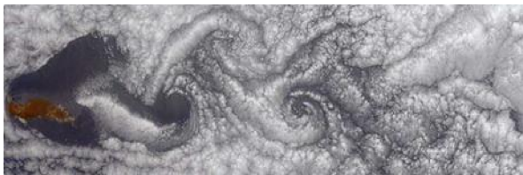
FIG. 4: Unstable manifold of a chaotic saddle traced out in a layer of marine stratocumulus clouds in the wake of Guadalupe Island on June 11, 2000, Courtesy of NASA, http://eosweb.larc.nasa.gov/HPDOCS/misr/misr_html/von_karman_vortex.html
